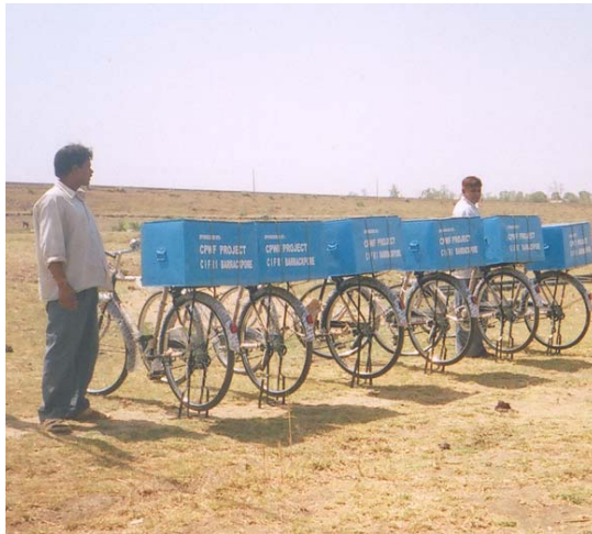
Photos 3.3. Left: bicycles fitted with iceboxes to improve quality of fish during transportation. Right: Market survey.
