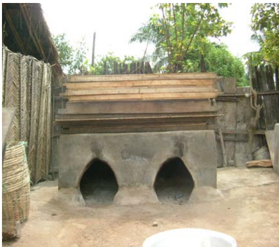
a. Chokor Smoker with a pile of trays to contain fish for smoking. Openings for fuel wood directly under fish.
