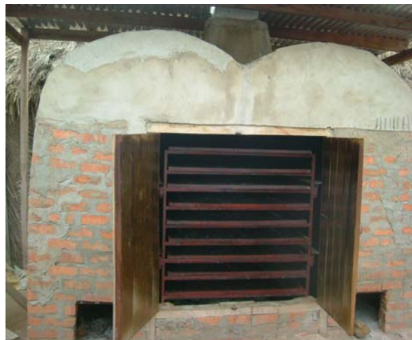
b. FRI-Smoker showing shelves as they would be positioned with Fish to smoke. Openings for fuel wood on side of trays holding fish
