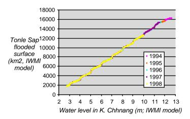
Figure 20: Computed flooded surface versus computed water level in K. Chhnang (flooding period)
