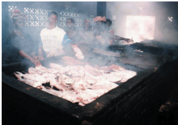
Cat fish smoking on the modified chorkor (bonga oven) in an improved conventional smoke house by the Fish Driers Association in Gunjur CFC.
