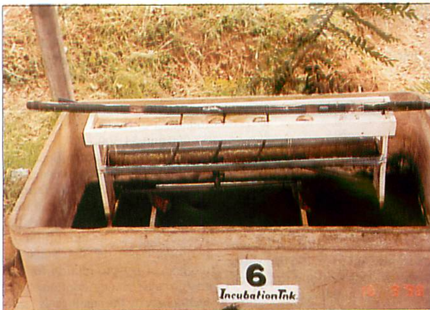
Fig. 1. Water re-circulating flow through system: incubation trays and tank with inlet and outlet pipes.
