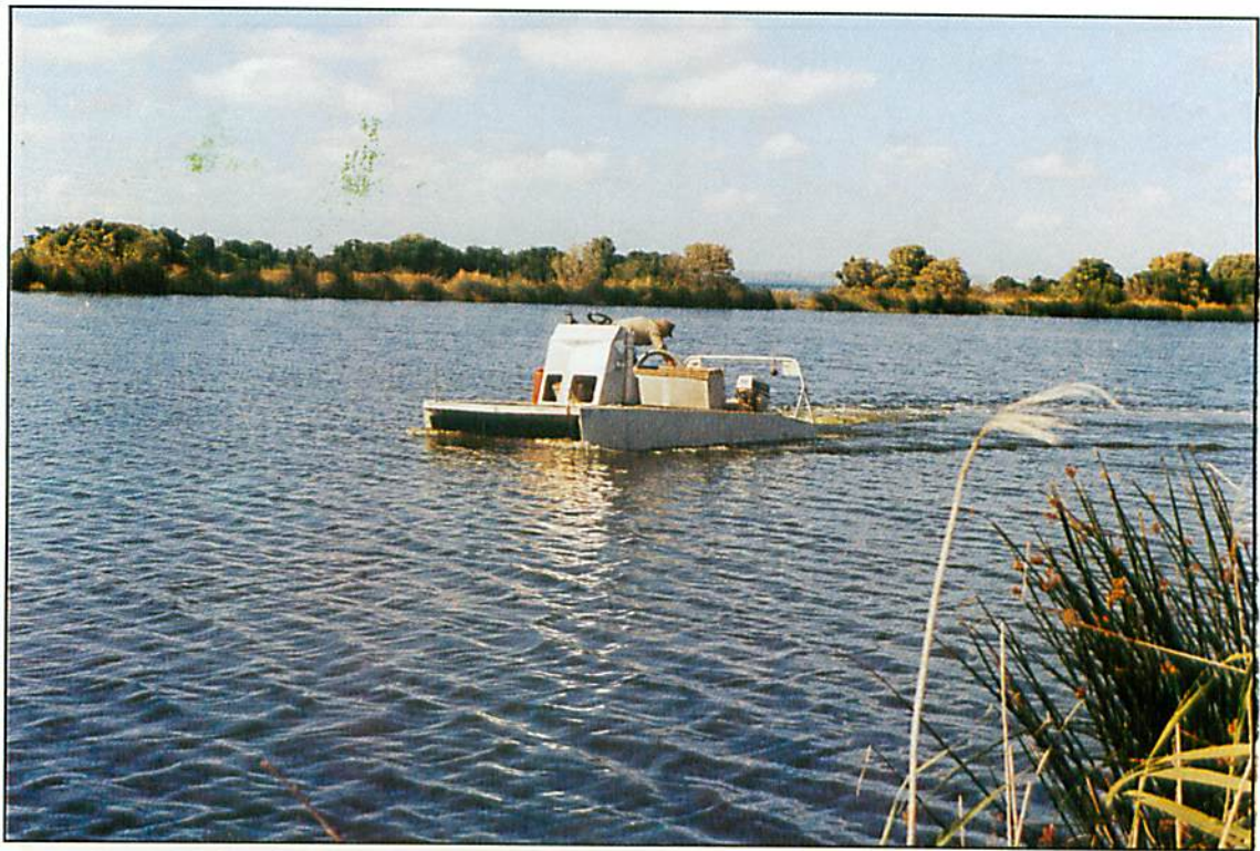
Harvesting zooplankton from WSTL using special harvester "Baleen". Water is filtered through screens to harvest the desired zooplankton.
