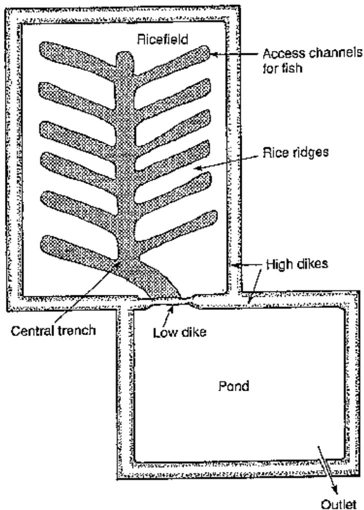
**FIGURE 4.** Rice-pond arrangement designed by two farmers. Rice field is sloped towards central trench and trench slopes toward pond.
