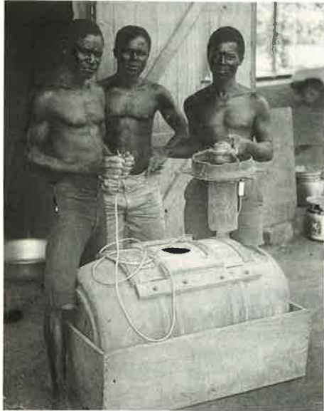
Fig. 1. Members of the Farmers Cooperative proudly showing an aerator (handmade from a used car fan) for live fingerling transportation.
