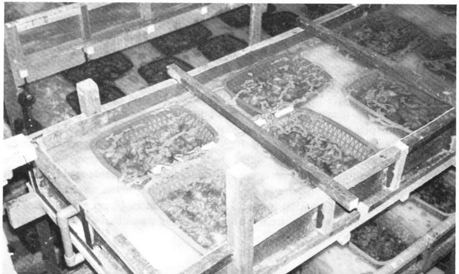
Holding tanks with sand/gravel filtering ( above ); looking down on raceways containing baskets of oysters ( below ) at Value Trading's depuration plant.
