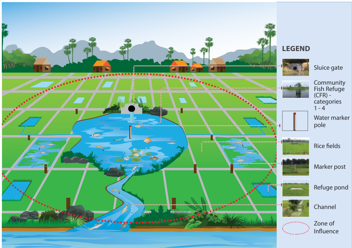
Figure 2: The main physical components of the Rice Field Fisheries / Community Fish Refuge system
