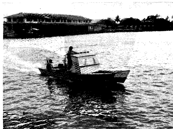
Fig. 2. Type B boat: a 28-ft alia with 25-hp outboard engine.
