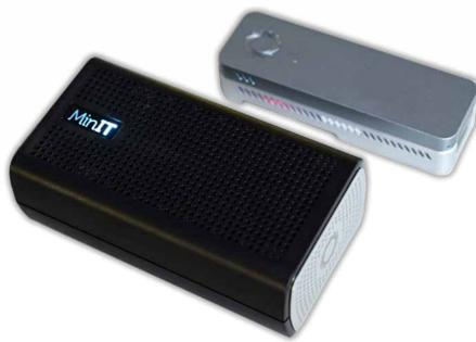
**Genomic sequencing** with **portable** Minion and MinIT devices from Oxford Nanopore Technologies
