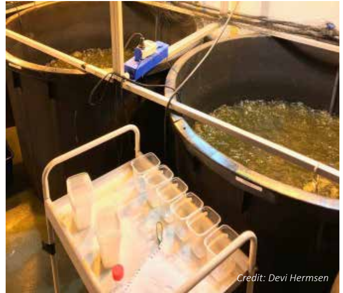
Simulated rearing mesocosm tanks at Wageningen University & Research (WUR), allowing a full nutrient budget to be made considering the cultured animals, water column, sediment and periphyton
