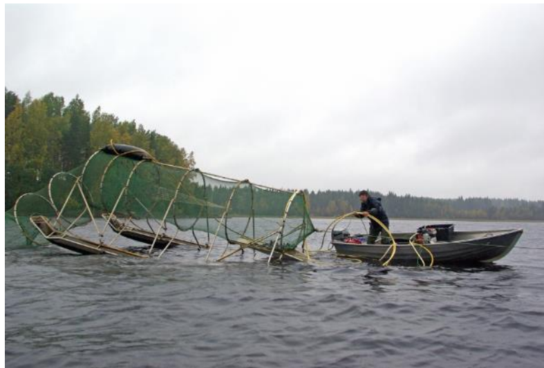
Photo 7.6. A fisher testing a new trap net technology for preventing seal bycatch.
