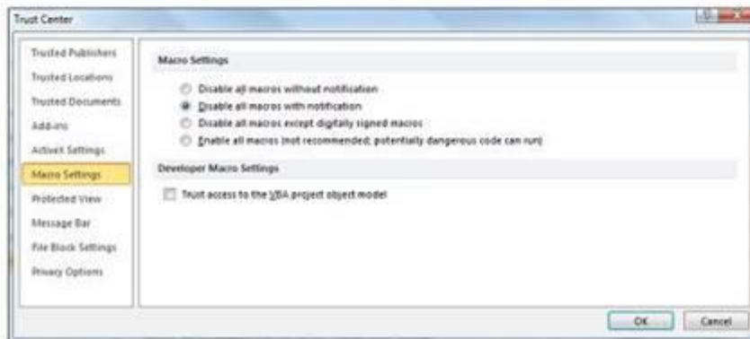
Figure 13. Procedure to access the check box to that states 'Trust access to the VBA project object model'
