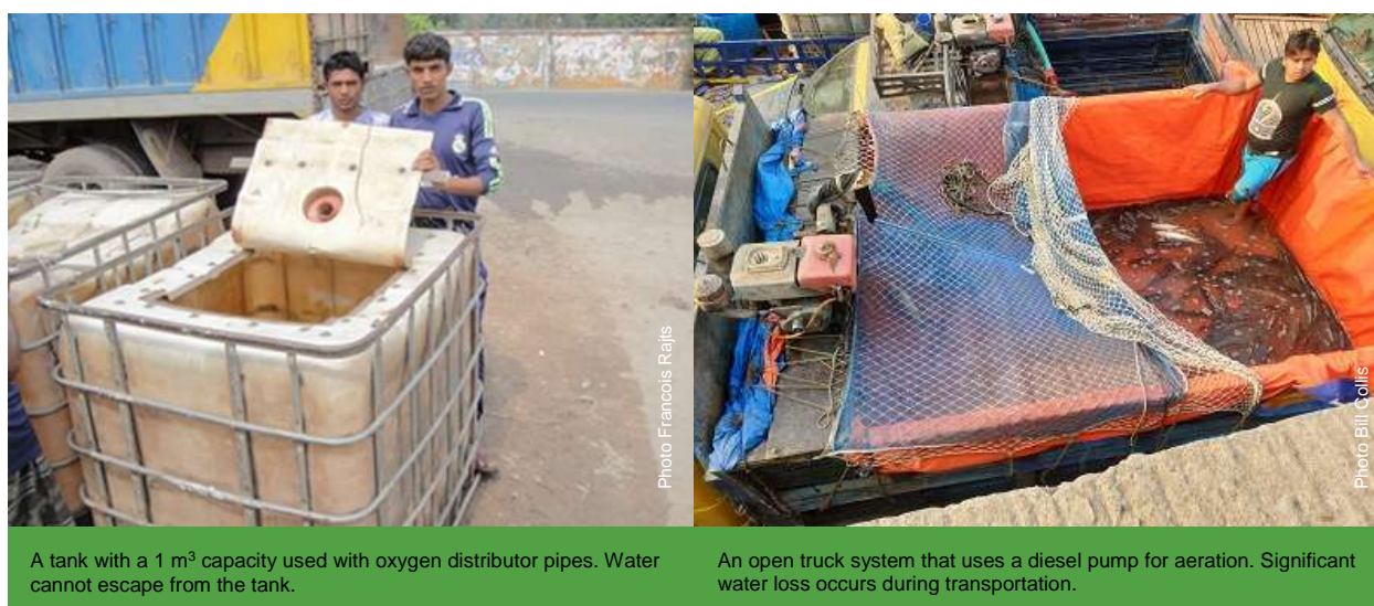
Plate 2. Two types of live fish transportation systems.
