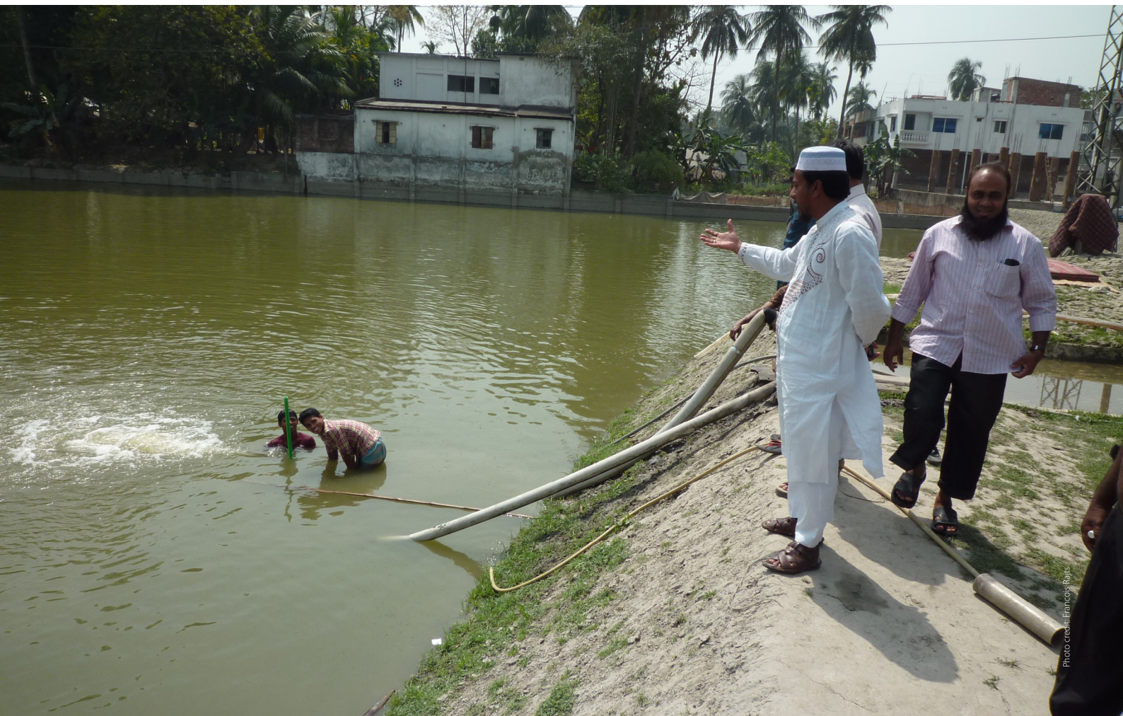
A venturi aerator significantly improved water quality and made year-round reproduction of several fish species possible in hatcheries in Jashore District.
