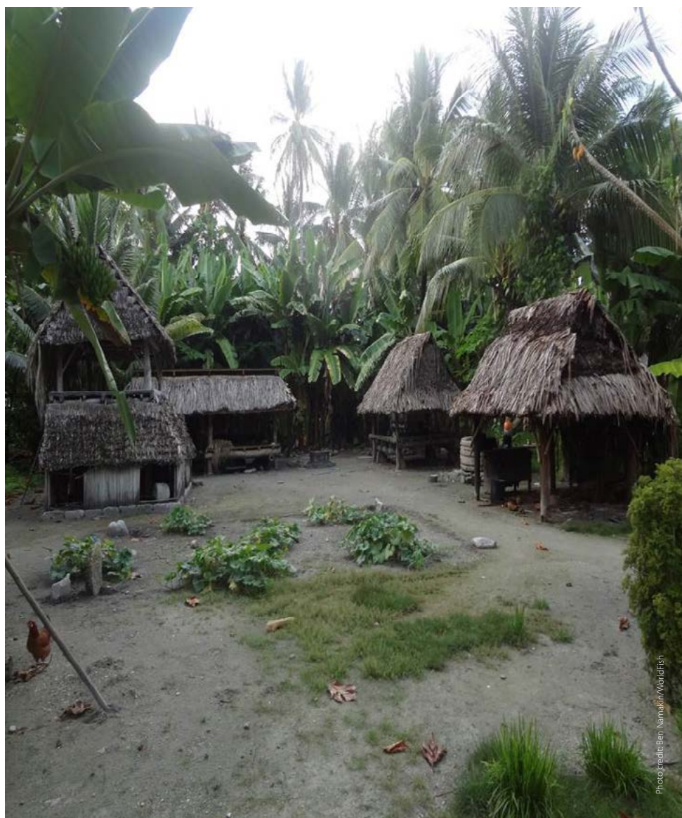
Figure 8. Traditional I-Kiribati houses, or buya , made of coconut and pandanus materials.
