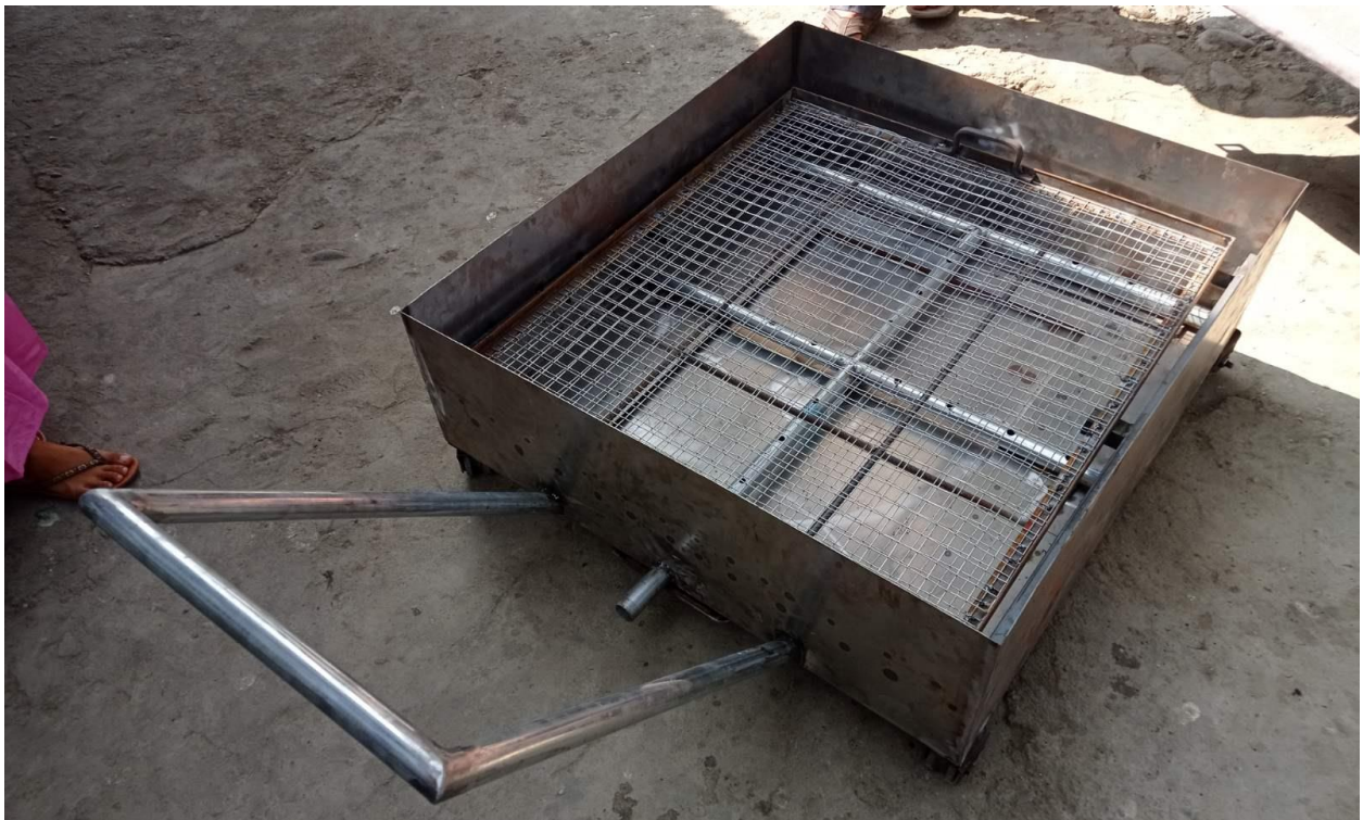
Figure 48: Fix the ember/charcoal tray just on the top of the air tubes giving enough space for fuelwood
