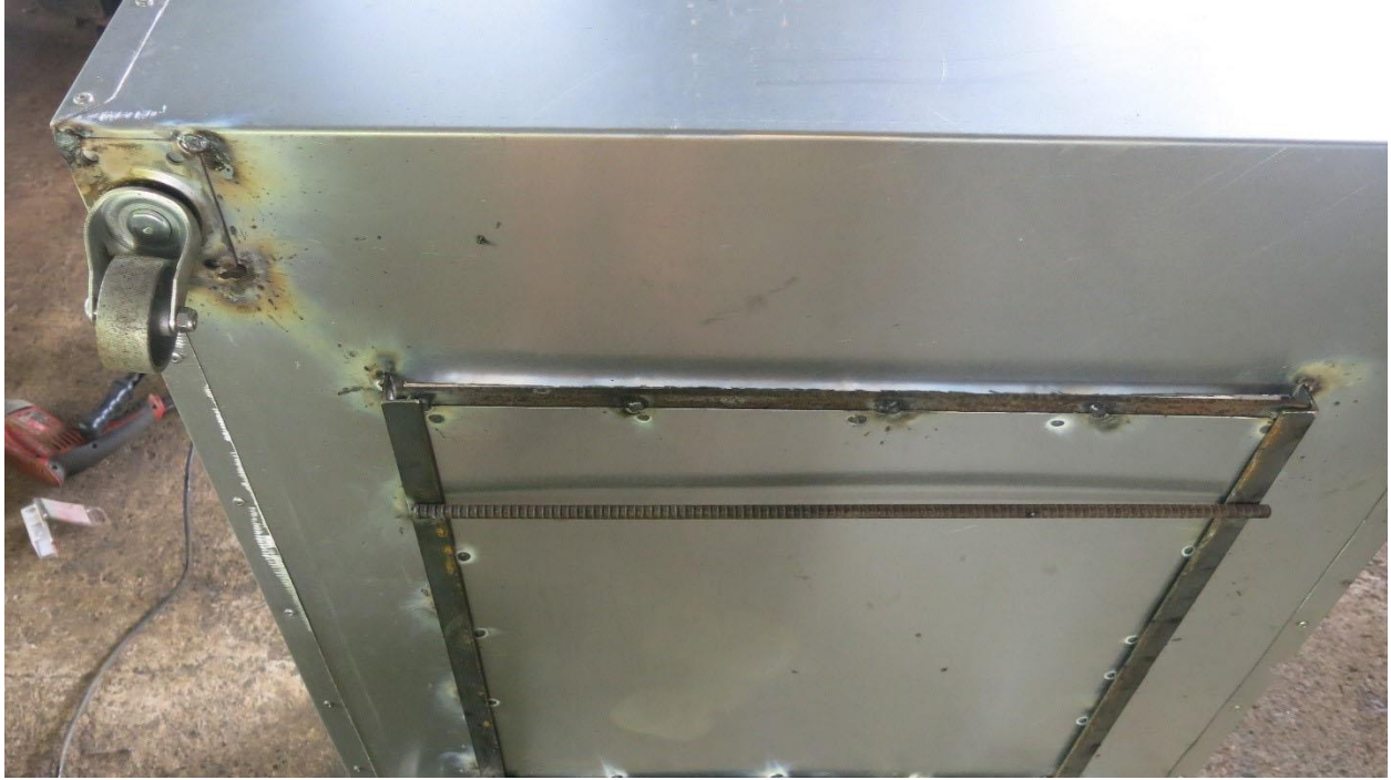
Figure 49: Bottom of the furnace
