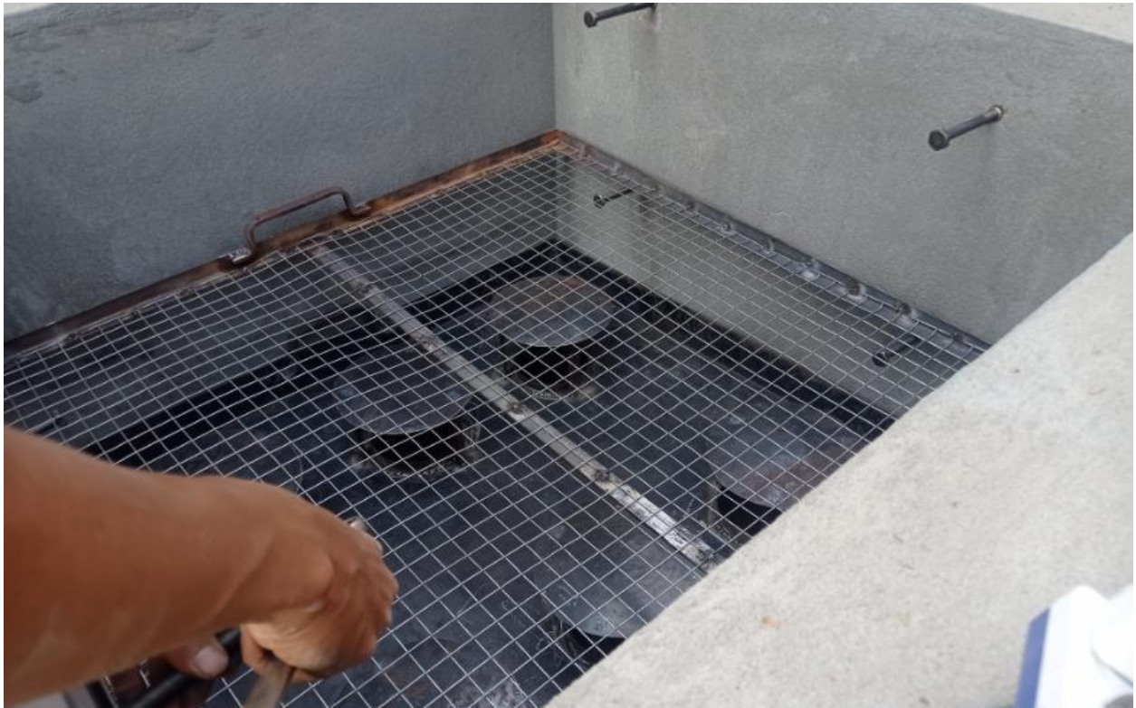
Figure 12: Check that there is enough space between the kiln chamber wall and the smoking racks / fat collection tray
