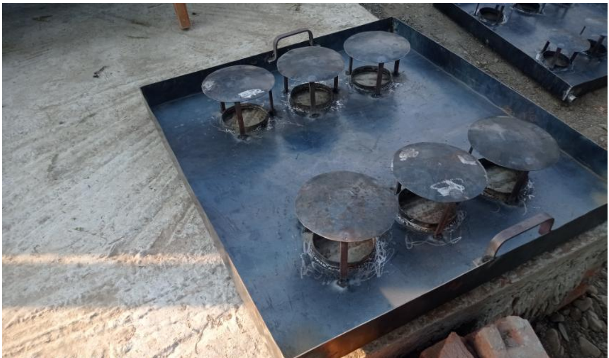
Figure 34: Fat collection tray with coned shaped cap
