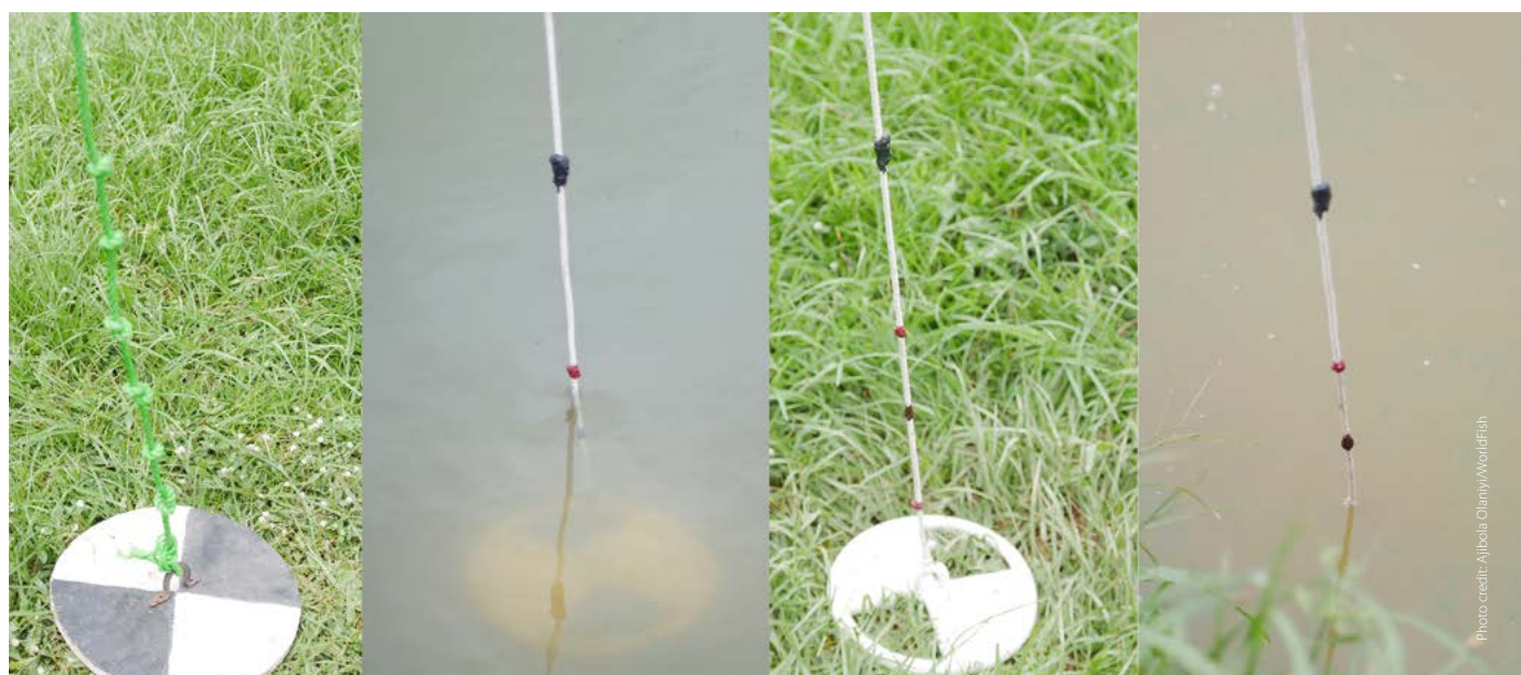
Plate 14. Monitoring pond turbidity.
