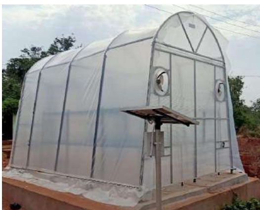
Low-cost Solar Fish Drier
