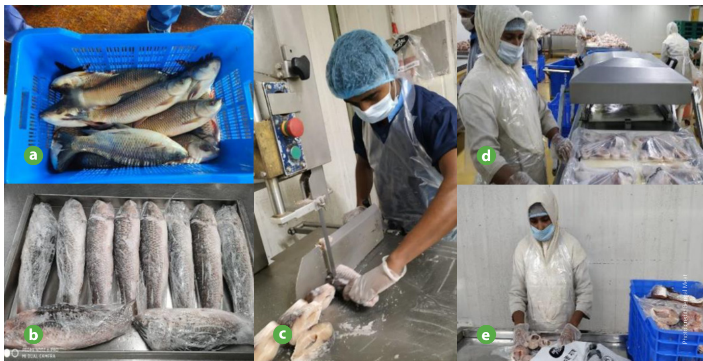
Plate 5. (a) Collected fish, (b) quick freezing, (c) cutting, (d) further packing and quick freezing, (e) final packaging.
