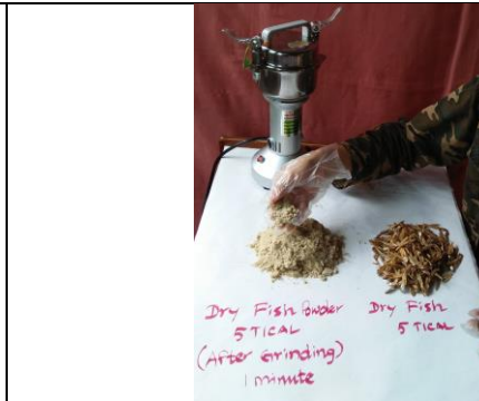
Photo 52. Multi-function electric grinder used to powder the dried SIS.
