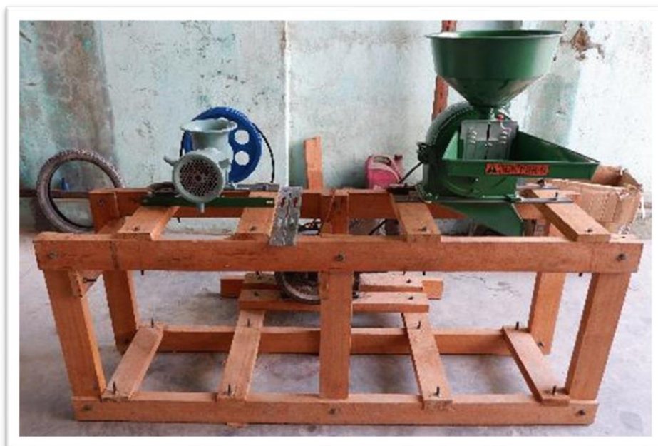
Photo 17. Feed mixing and pelleted fish feed milling equipment.
