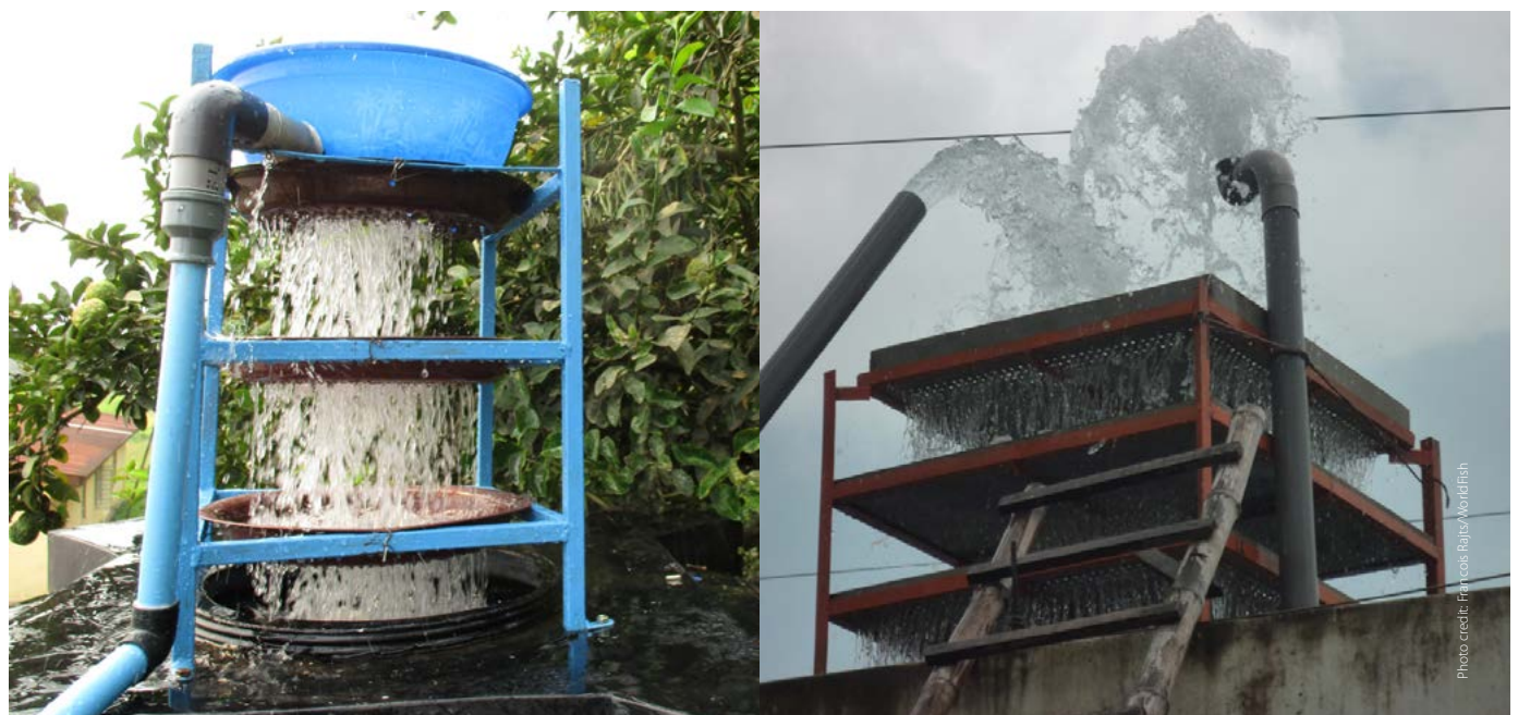
Plate 2. Aeration tower in a small hatchery in Sierra Leone (left) and an aeration tower (designed by F. Rajts) for a large hatchery in Bangladesh with high levels of carbon dioxide (right).
