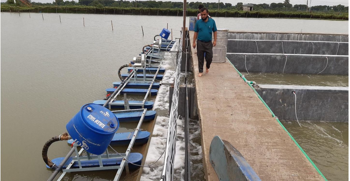
Provision of continuous water flow into the production cells of IPRS by Afil Aqua Fish Ltd.
