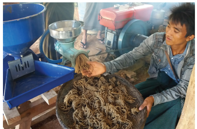
Testing the solubility of farm-made sinking pellet feed made from various small machines in the Ayeyarwady Delta.
