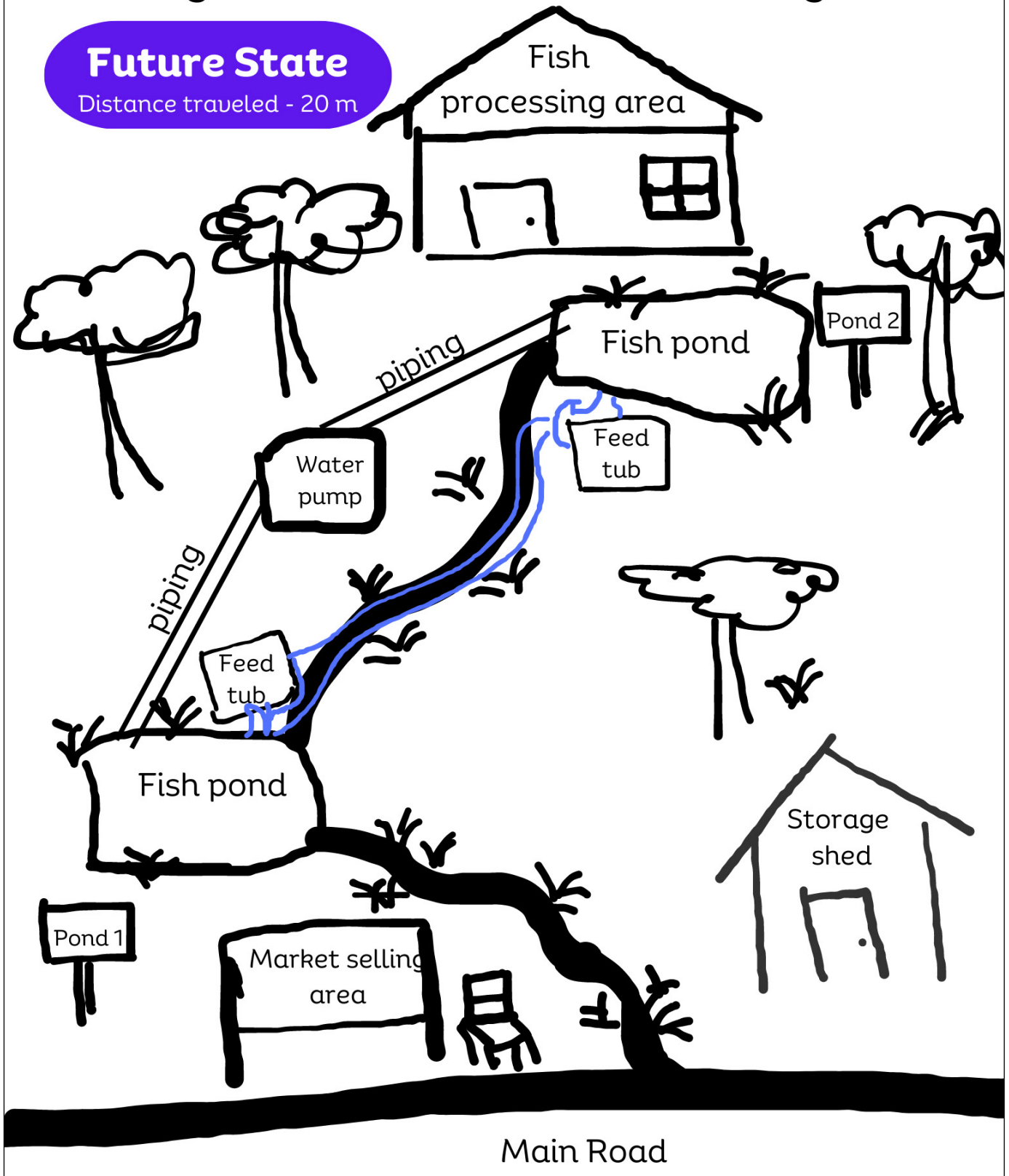
Figure 20. A spaghetti diagram of the future state or process movement of Mary's farm.
