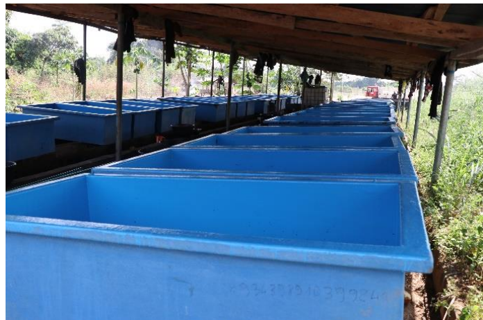
Nursery Glass Fibre tanks with no inlet
