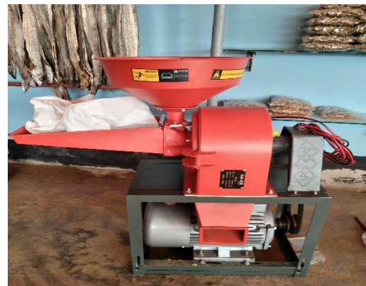
Fig-23: Safe dry fish powder making machine (P.C. Mahbub Alam, BDO)
