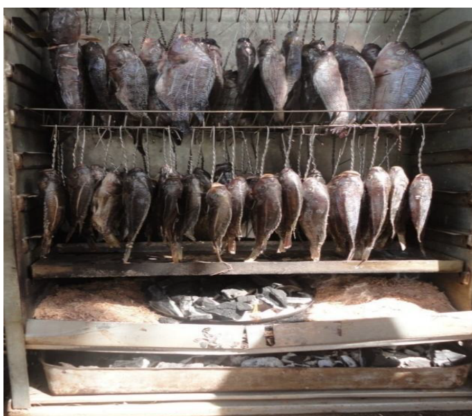
Figure 15. Improved fish smoking kiln (courtesy of Dr. Domitila Kyule of the KMFRI).
