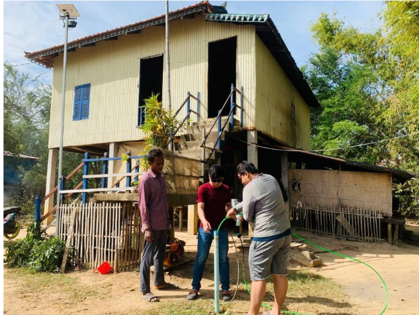
Figure 3: Primary investigation and measurement of the static groundwater level
