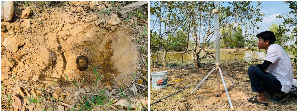
Figure 6: Soil data collection and permeability test activities
