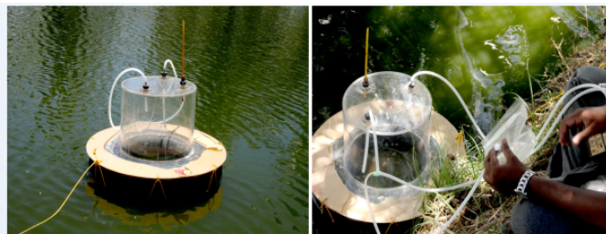
Figure 4. Sampler for collection of GHG samples from aquatic systems.
