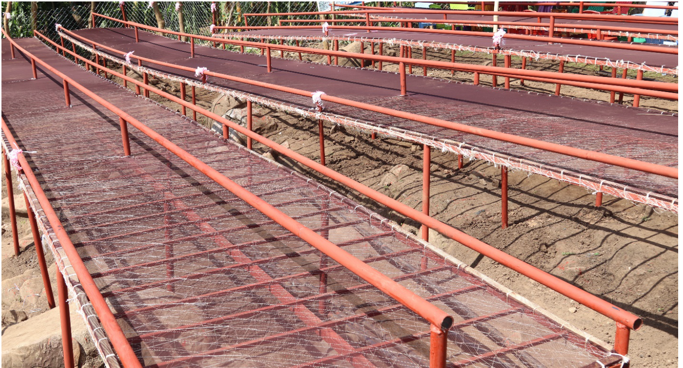
Figure 4. Modern drying racks made of steel, constructed to improve the processing of dagaa for women and sustain in the climatic shocks.
