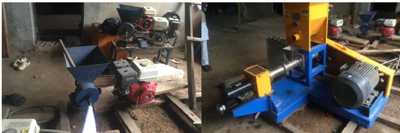
Plate 9. Fish feed extruder at Flourishing Centre Fish and Agro Farms.
