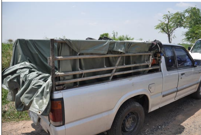
FIGURE 6 Live tilapia transporting equipment (modified truck with plastic sheet and oxygen tank) owned by a group of tilapia farmers in Chonburi Province
