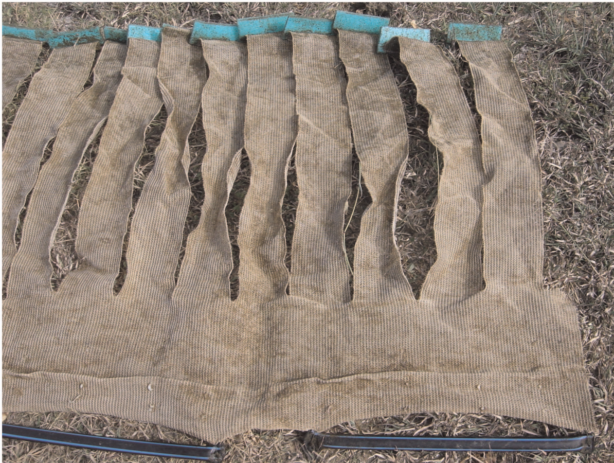
Figure 1. Stripped shadecloth unit. Photograph of the end of a stripped shadecloth unit used to increase the surface area of mesh inside fine-mesh enclosures. The sand-filled polypropylene tubes at the bottom of the photograph weigh down the woven polyethylene fabric while the foam pieces at the top kept the strips upright in the water. doi:10.1371/journal.pone.0064103.g001
